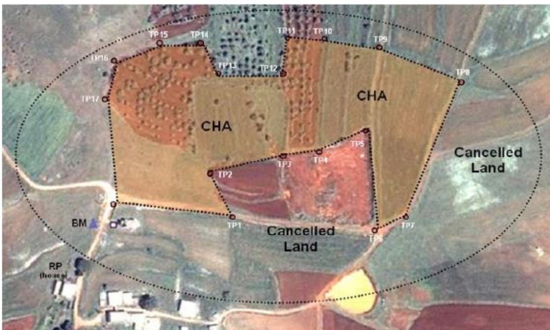
Figure 2 – This picture illustrates a possible conclusion of an initial non-technical survey. Based on further evidence the area outside the CHA has been cancelled and the CHA has been marked, for mapping purposes only and not physically on the ground, with a Reference Point (RP), Bench Mark (BM) and Turning Points (TP).
